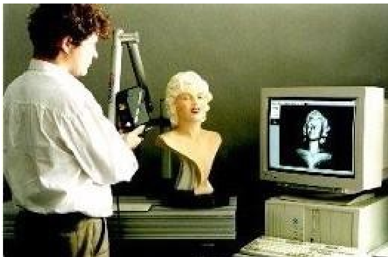
Slika 2.5 3D skener ModelMaker (Ebrahim, 2011)
