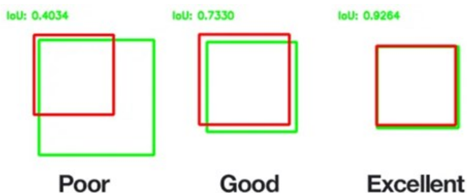
Slika 2.8 Prikaz Intersection over Union (IOU) (Dey, 2023)
