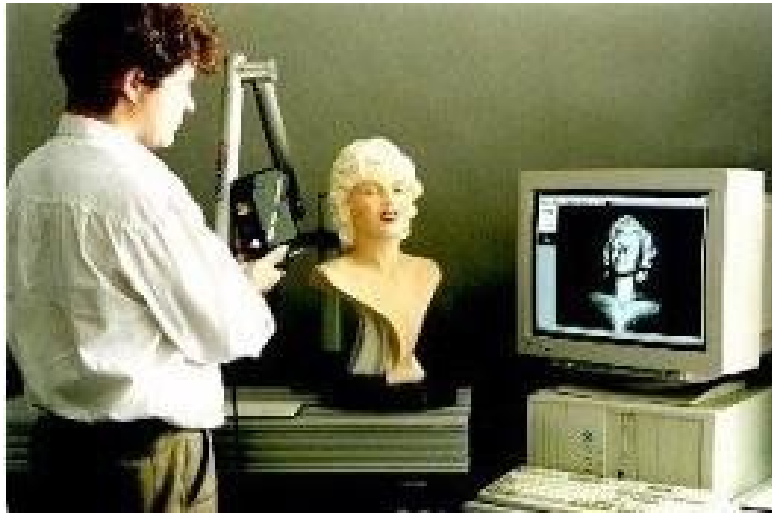
Slika 2.5 3D skener ModelMaker (Ebrahim, 2011)
